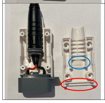
Put this subassembly in the charger housing connector (3). The housing (1) slides in at the red circled position and adapter (2) at the blue circled position in housing (3).
