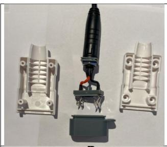
Connect the battery connector to the quick plug adapter (2). Only possible in one way.
