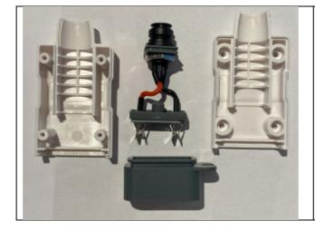
Open the adapter connector. Only 4 main components are part of it (see BOM).
